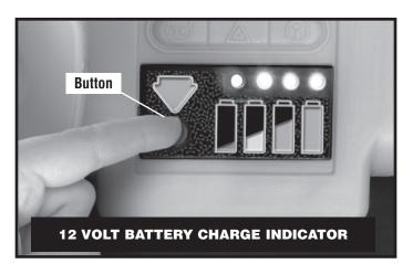
**IMPORTANT!** Do not press the 12 volt battery charge indicator while the vehicle is moving.
